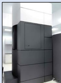
Titan Krios G3i 300 kV cryo-TEM
